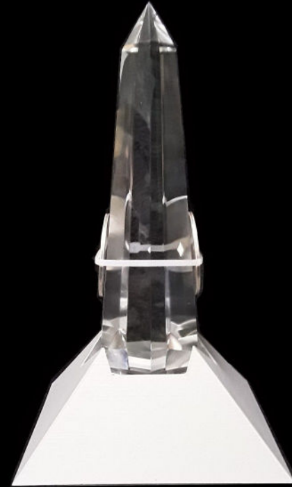
2 configurations to support the crystal with pure silver electrodes
